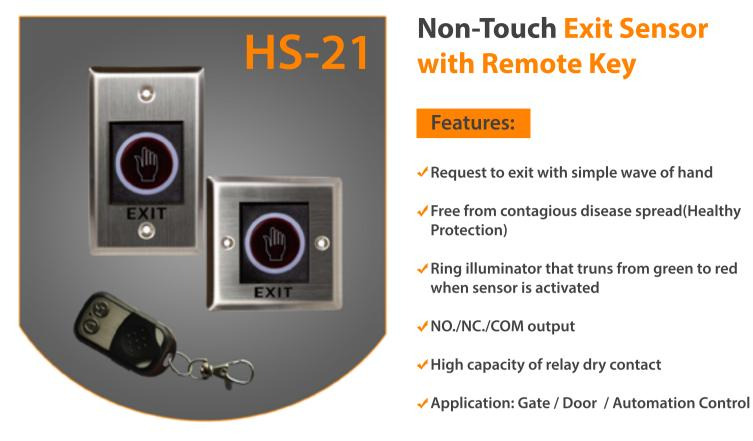
HS-21 series exit switches adopt optical infrared technology which requires no physical contact, and by the means of 433 MHz RF transceiver technology, the wireless key could unlock the door remotely after configured with HS-21. It is more convenient to open the door for visitors from a faraway place.
